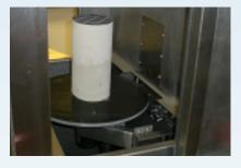
Catalytic converter in x-ray chamber
