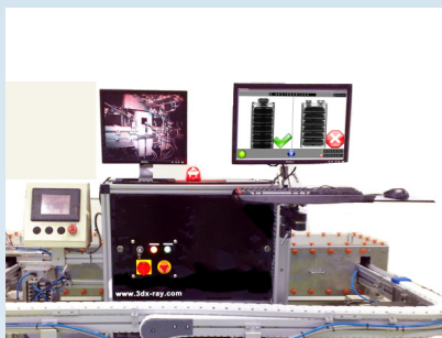
Battery inspection installation
