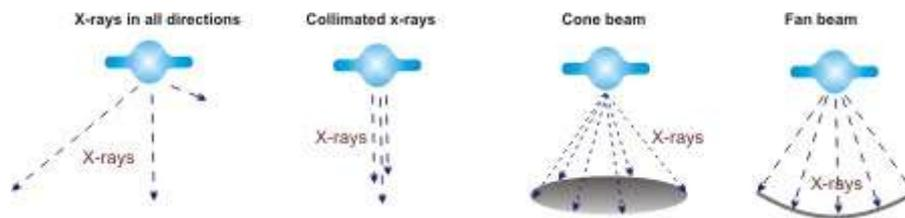
When the x-ray beam enters an object it will interact with the material in one of three basic ways. It could pass through it completely unhindered, it may become totally absorbed or it may in some way interact with the material and be scattered, that is leave the material at a different angle and energy to that of the incident primary beam. The proportion of x-rays that pass through, are absorbed or are scattered will be dependent on the energy of the x-rays and the material they pass through.
