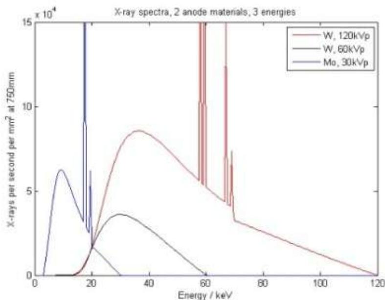
A number of parameters affect the characteristics of the x-rays produced by an x-ray tube and determine the spectrum. The characteristics affected are:
