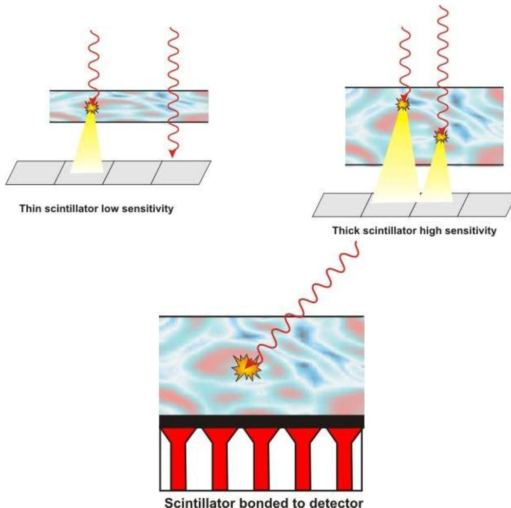
Different types of scintillators are used depending on the energy of the x-rays to be detected. The scintillators can also be used in different configurations. In one possible configuration the scintillator is bonded directly onto the electronic device such as the CCD or amorphous silicon panel which increases the collection efficiency.
