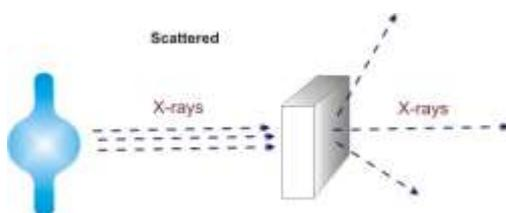
In general scattered x-rays are created by any material that the x-ray beam hits, the target, air, x-ray shielding such as steel or lead, and travel in all directions. As a result, any x-ray system will produce x-rays from a number of points and surfaces. These scattered x-rays are important,
