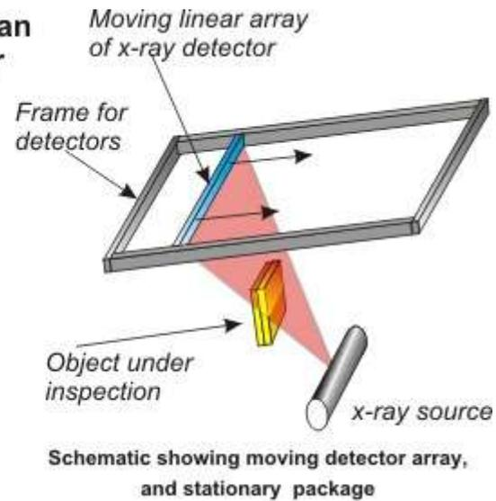
Producing an image using a line scan may use a thin curtain of x-rays to illuminate the detector array. As the object passes through the inspection area it is illuminated by the x-ray curtain and the resultant line image formed on the detectors is continuously read by the computer, building up a complete image of the object line-by-line. This technique also reduces the x-ray exposure to the object being inspected by around 98%.
