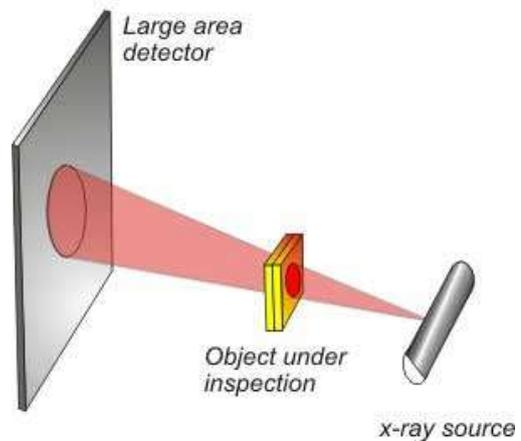
The different configurations are suitable for different applications. For example, in baggage
