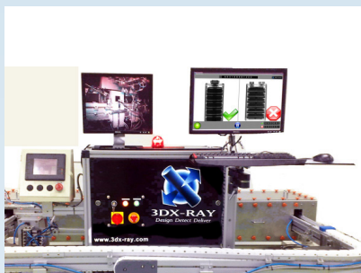
Battery inspection installation
