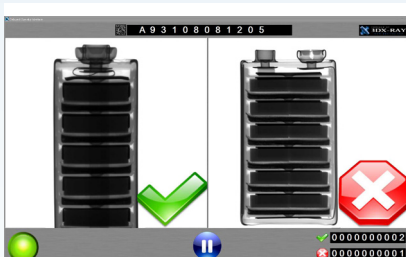
Real time pass/fail display
