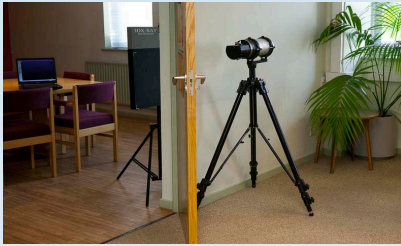
FlatScan-TPXi deployed to x-ray through wall using tripods
