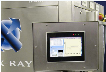
Results graph indicating pass/fail for profile analysis and coating depth analysis
