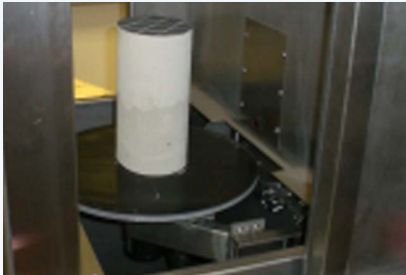
Catalytic converter in x-ray chamber
