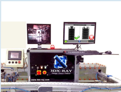
Battery inspection installation
